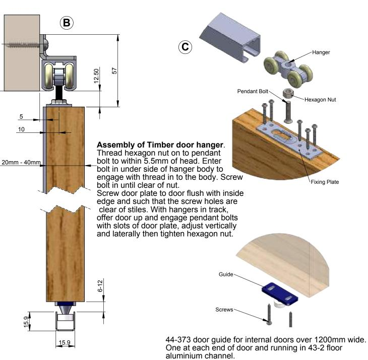
CAUTION: Do not wind the Pendant Bolt all the way past the top of the Hanger, as this will stop the system from working properly
